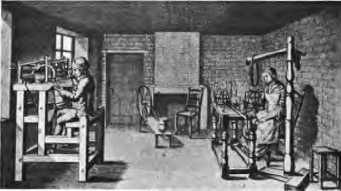
FIG. 64.—The Stocking Trade (18th century). To the left, a Stocking Maker. To the right, a Woman working the Lyons Spinning-Jenny.
